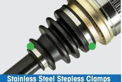
Provides improved clamping force on the TPE boot to create a tighter, more reliable 360° optimum seal even in the most extreme temperatures.
